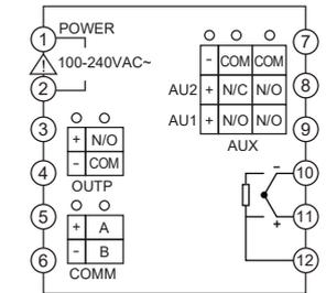
**Note 1:** Dimension D61 instruments does not support 0~1V and above linear voltage input. Instead, 0~1V signal can be converted to 0~100mV by external voltage divider while 4~20mA can be converted to 20~100mV by connecting a 5 ohm resistor in parallel, then be inputted from terminals 11+ and 10-.
