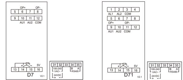
**Note 1:** Input 0~5V/1~5V input from 16+, 15-. 100mV below input from 14+, 15- 4~20mA with 250ohm shunt resistor converted to 1~5V, input from 16+, 15-
