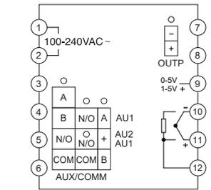
**Note1:** Linear voltage signal with its range below 100mV can be inputted from terminals 11+ and 10-, 0~1V and 0~5V signal can be inputted from terminals 9+ and 10-;
