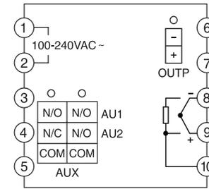
**Note 1:** Dimension D2 instruments support neither 0~5V nor 0~5V linear voltage input. Instead, 0~5V or 1~5V signal can be converted to 0~100mV or 20~100mV respectively by external voltage divider while 4~20mA can be converted to 20~100mV by connecting a 5 ohm resistor in parallel, then be inputted from terminals 9 and 8.
