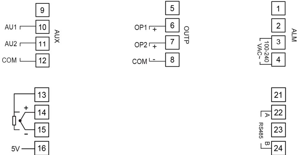
**Note 1:** 0~5V/1~5V and above voltage signals are input from 16+, 15-, 0~100mV and below signals are input from 14+, 15-; 4- 20mA linear current input and 250 ohm resistor into 1-5V, then input from 16+, 15-.
