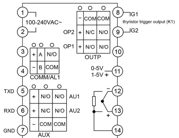
■ The wiring diagram of E7 panel instrument (22.5X100mm) is as follows:
