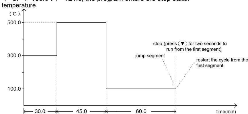
The platform mode only needs to set the temperature and constant temperature time. It does not need to set the temperature rise process. As shown in the figure above, the platform mode can be set to skip, stop, cycle, etc. The above settings are actually listed as stop.
