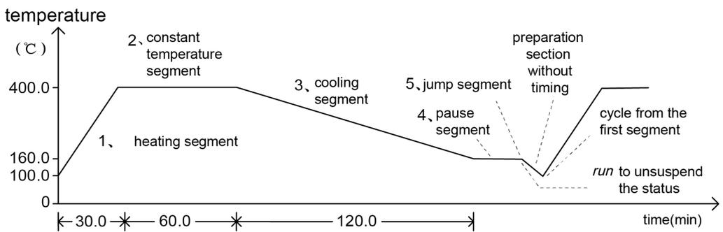
The advantage of using temperature-time programming method is that the slope setting range of temperature rise and drop is very wide. The heating and constant temperature sections have a unified setting format, which is convenient for learning. Besides, it is more flexible to set curve, and possible to set a continuous heating section (for example, use a heating section with different slopes to approximate functional heating), or a continuous constant temperature section as well.
