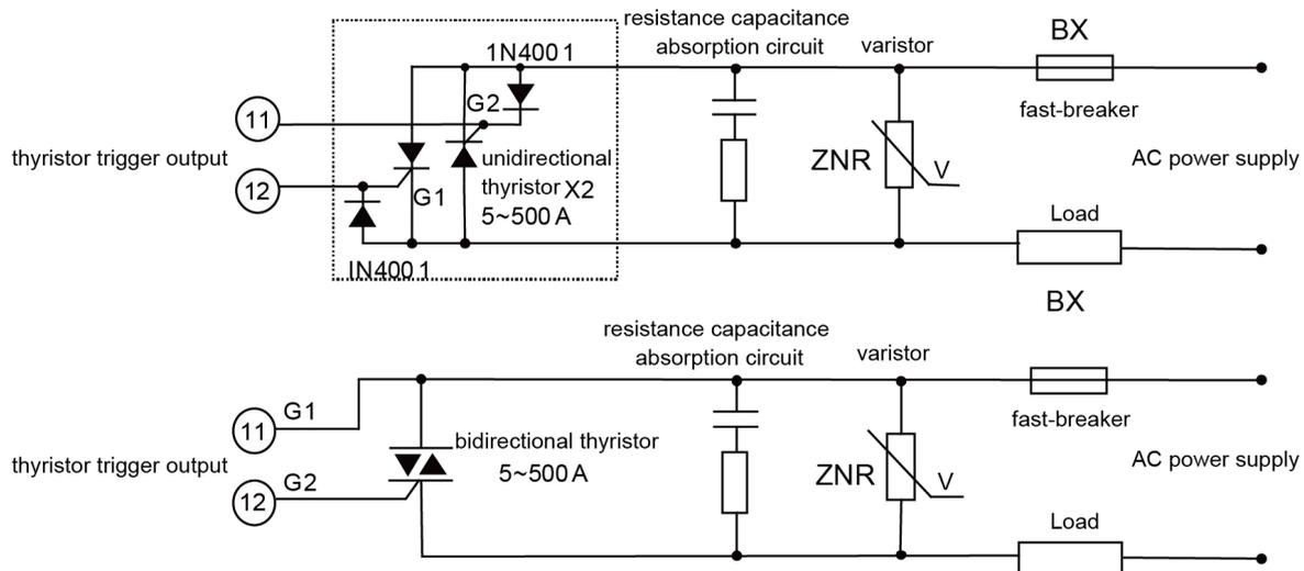
Note 1: Resistor-capacitor absorption and varistor must be added when phase-shift trigger is used to improve possible harmonic interference.
