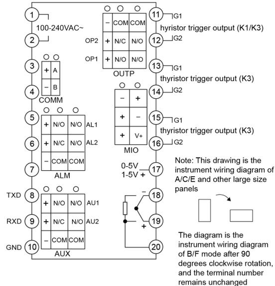
■ The wiring diagram of D-type panel instrument (72mmX72mm) is as follows:
