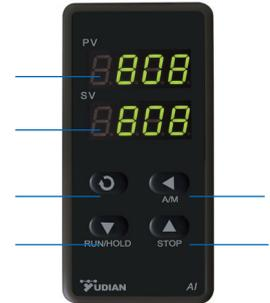
Parameter setting method: When the parameter lock is not engaged, press and hold the (Set) key for about 2 seconds, then release it when the parameters are displayed. Next, press the (Set) key again, and the instrument will sequentially display parameters, such as loop 1 input specification InP1, parameter lock Loc, and others.
